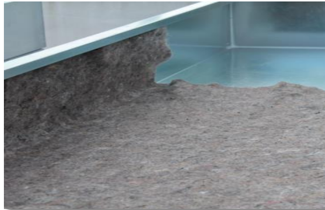
Figure 13. The protection and retention mat NativeScapeGR project
