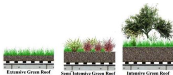
Figure 8. Different type of green roofs ( https://www.buildup.eu/en/learn/ask-the-experts/which-are-different-types-green-roofs ).
