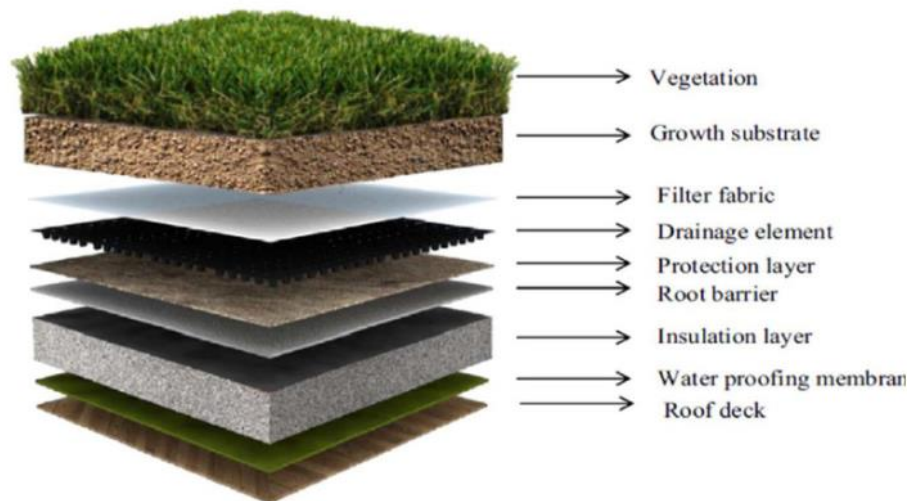
Figure 9. Components of the green roof structure ( https://www.buildup.eu/en/learn/ask-the-experts/which-are-structural-components-form-green-roof/ ).
